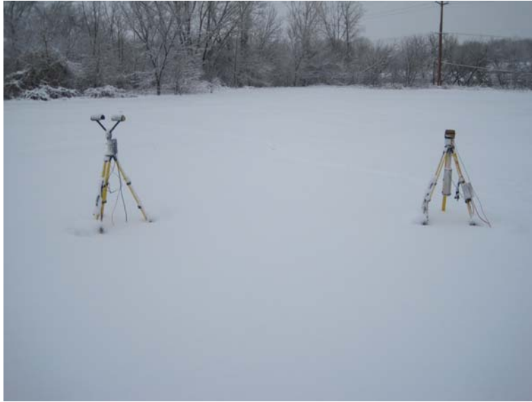
Fig. 11. Image of the Parsivel disdrometer and rain gauge / field mill looking toward 20 deg from the MIPS trailer.
