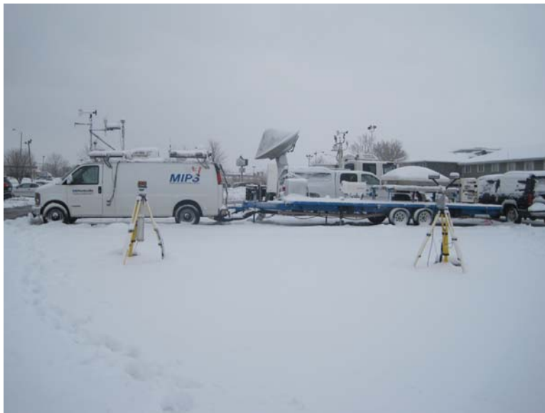
Fig. 12. Image of the MIPS taken about at 1600 UTC on 9 December. The view is towards 200 deg. The Parsivel disdrometer (right) and rain gauge / field mill (left) are in the foreground.
